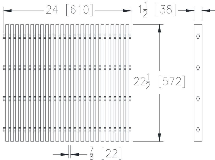
**GG GRATE ENGINEERING SPECIFICATION:** The Zurn P817-GG-24X24 Slotted Grate, Fiberglass, 24 inches wide by 22-1/2 inches long, weighing 15.29 lbs. The grate has an open area of 236.25 square inches, DIN Rating of A and ANSI Rating of Light-Duty.
